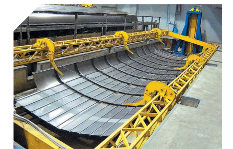
Rotator for car roof sheathing welding
