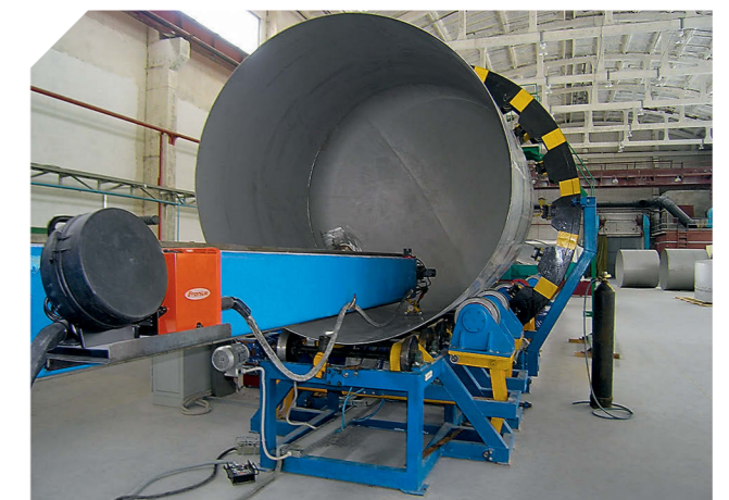
Internal seam welding
