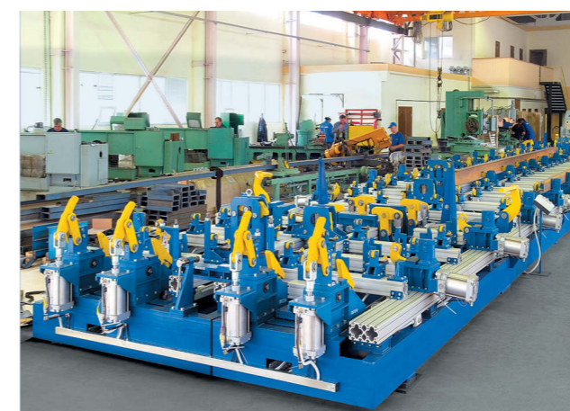
Multipurpose stand for passenger car underframes assembly
