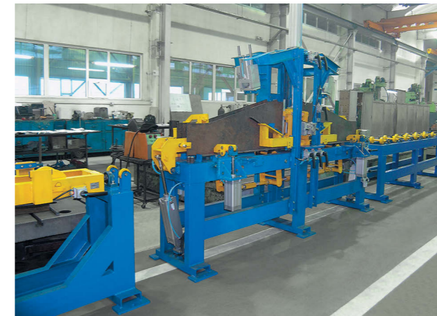
Assembly of freight cars intermediate bearers
