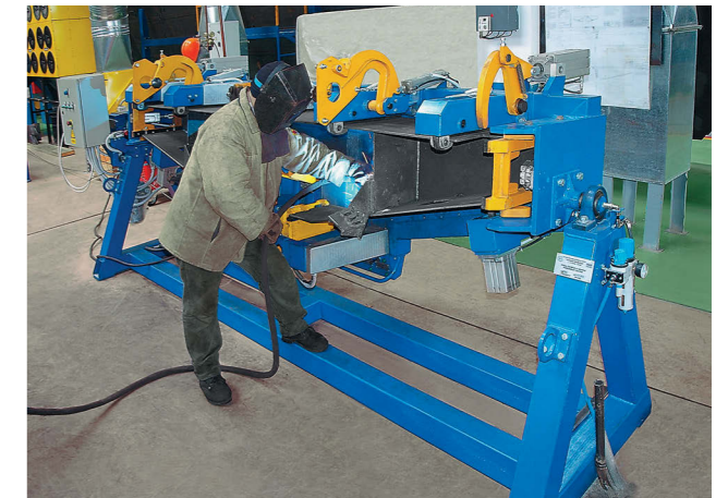
Assembly of freight cars intermediate bearers
