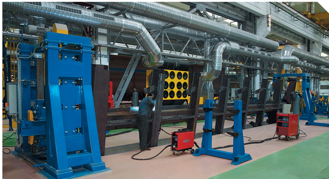
Rotator with lifting supports, load capacity - 15 t
