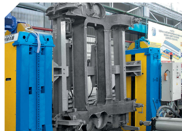
Rotator with lifting supports, load capacity 4 - t
