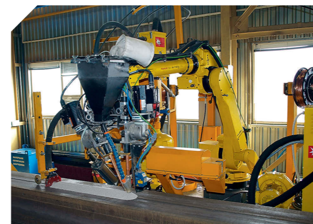
Laser seam tracking system META
