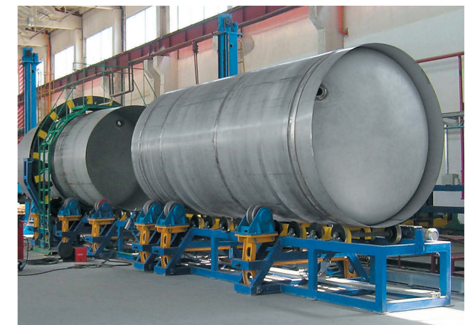
Vessel assembly and welding line
