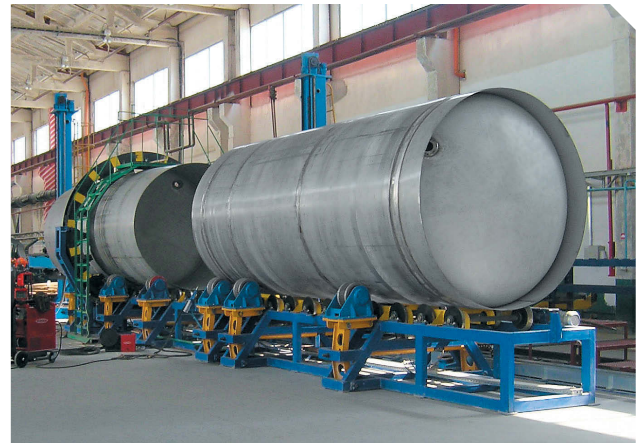
Line for assembly nad automatic welding of vessels
