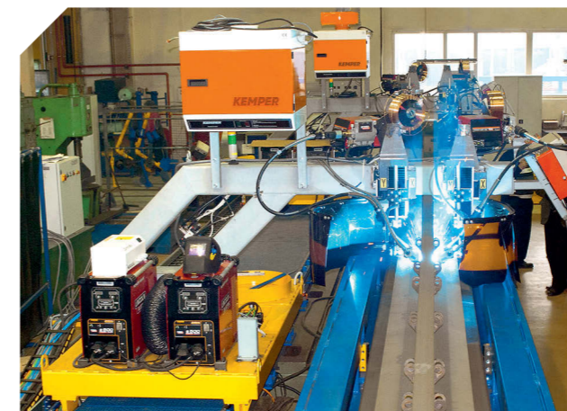
Simultaneous welding with two torches
