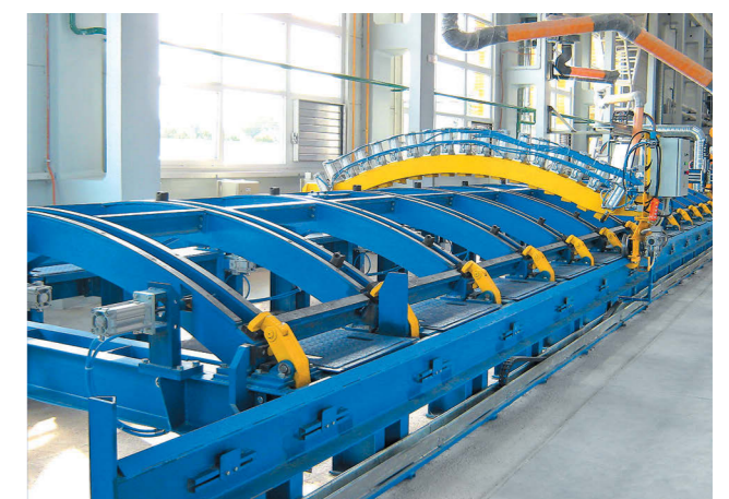
Box car roofs assembly stands
