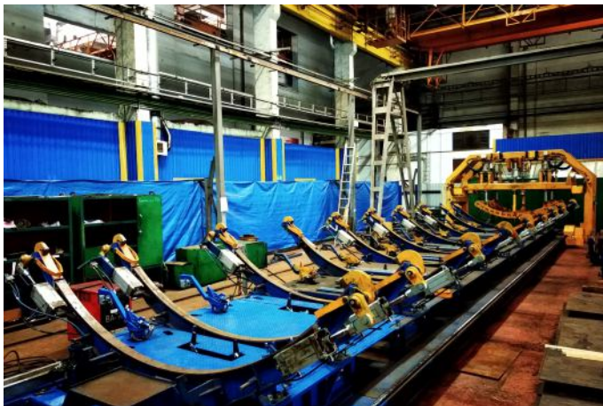
Multipurpose stand for hopper cars roof assembly and welding
