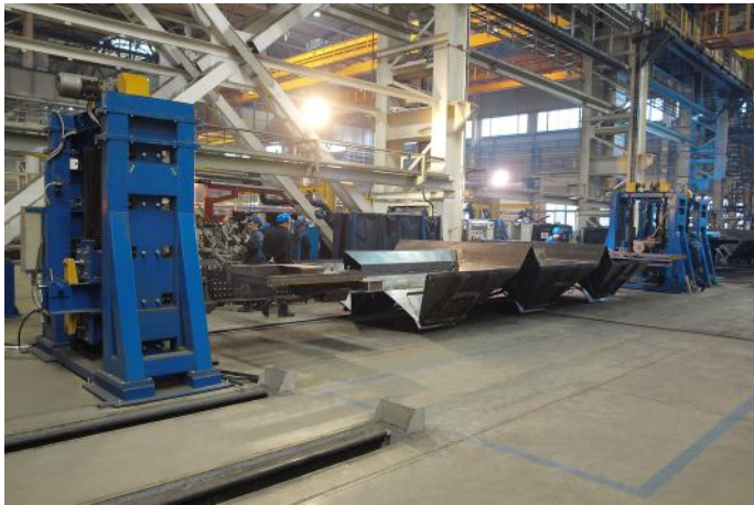
Headstock and tailstock positioners, load capacity 15 tons
