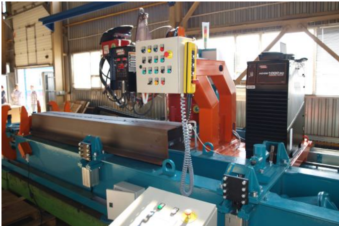
Automated welding fixture for center sills of tank wagons
