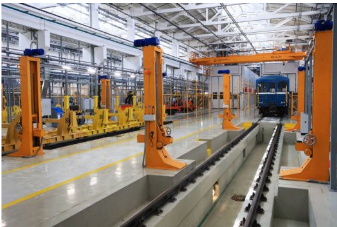
Stationary jacking unit — 60 ton capacity
