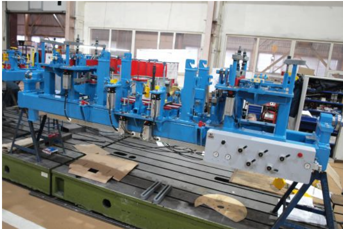
Assembly station for railway bogie frame beams
