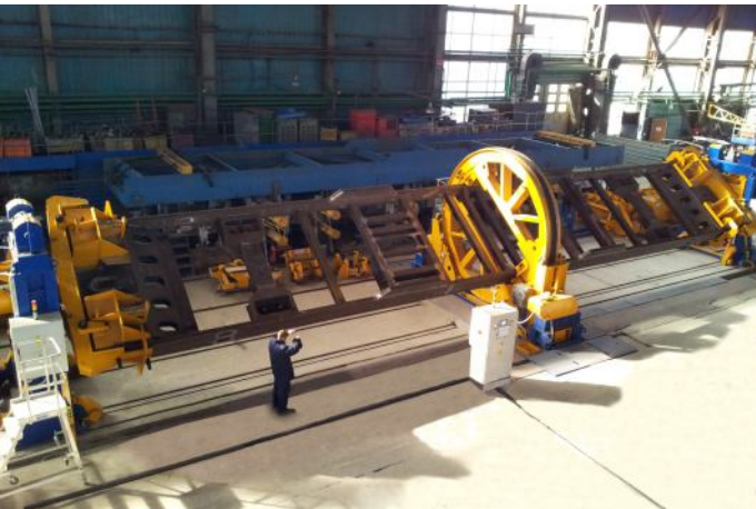
40-Ton frame positioner for electric locomotives
