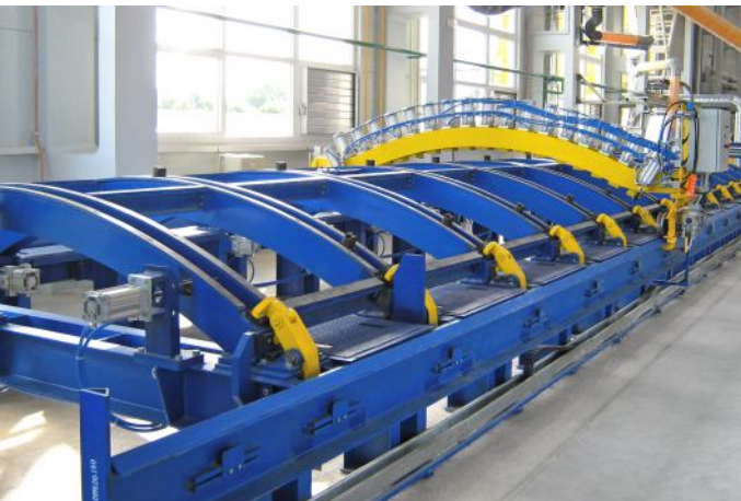
Multipurpose stand for assembly of boxcar roofs
