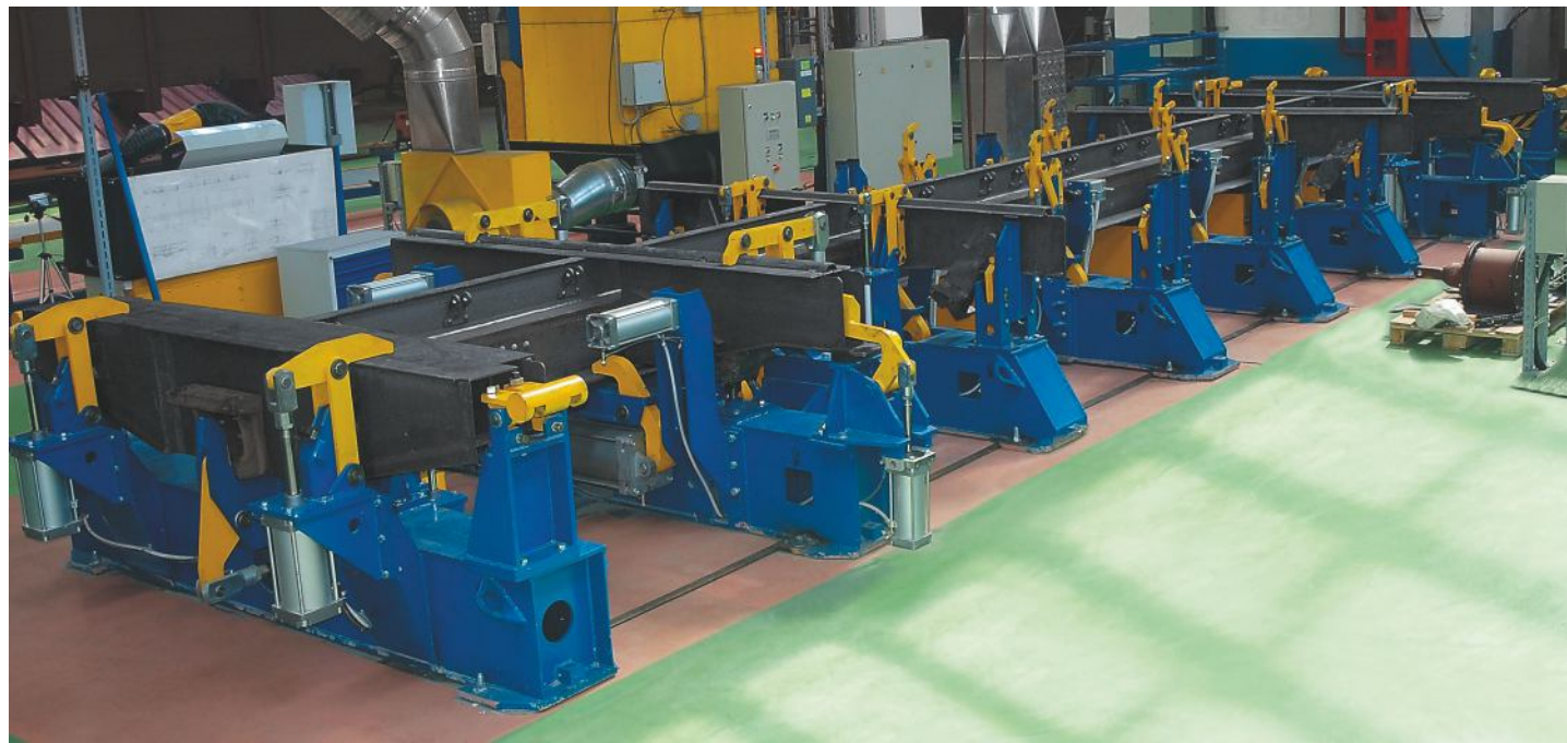
Gondola wagons underframes assembly and welding stand
