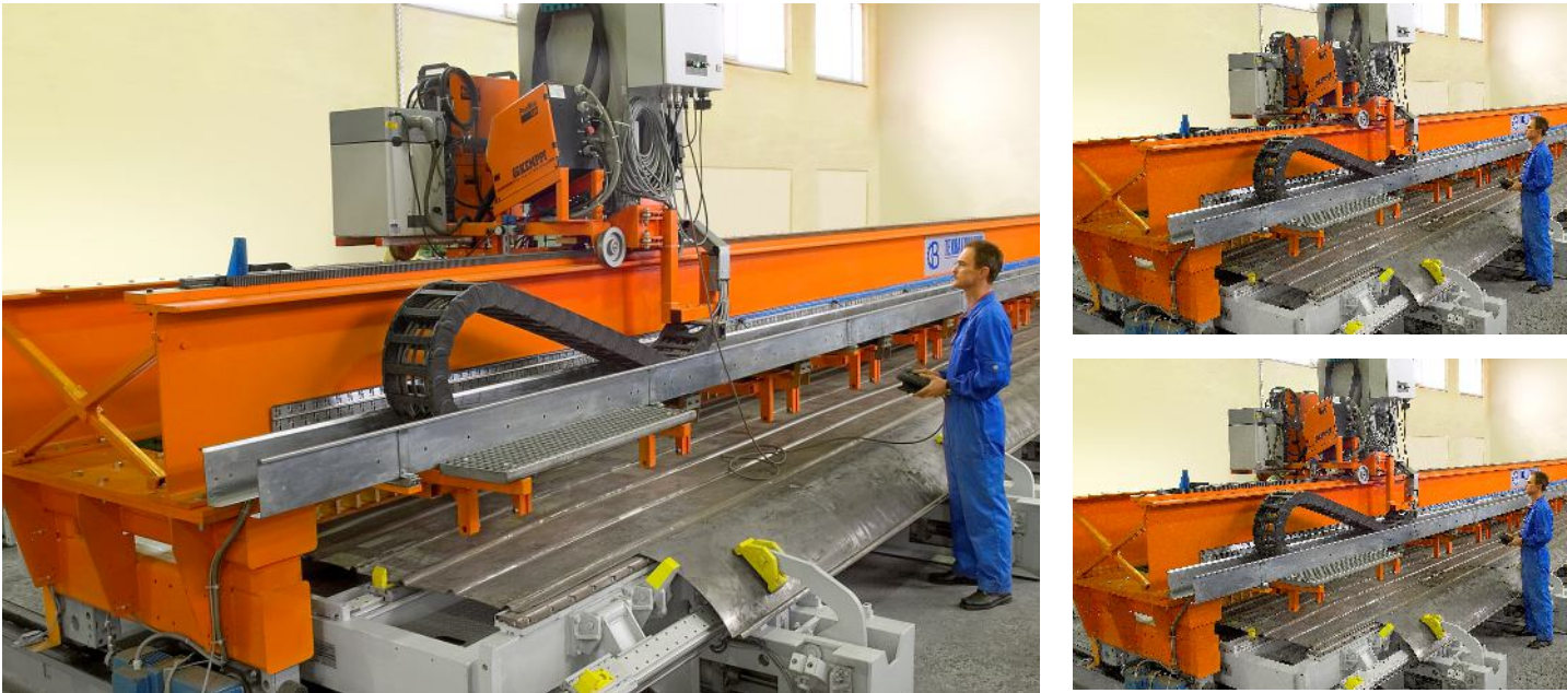
Multipurpose automated welding station for metro wagon roof panel sections
