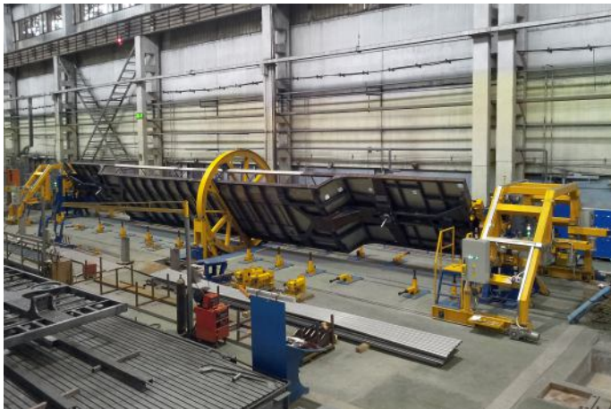
Positioner stand for floor deck welding and under-carriage equipment assembly
