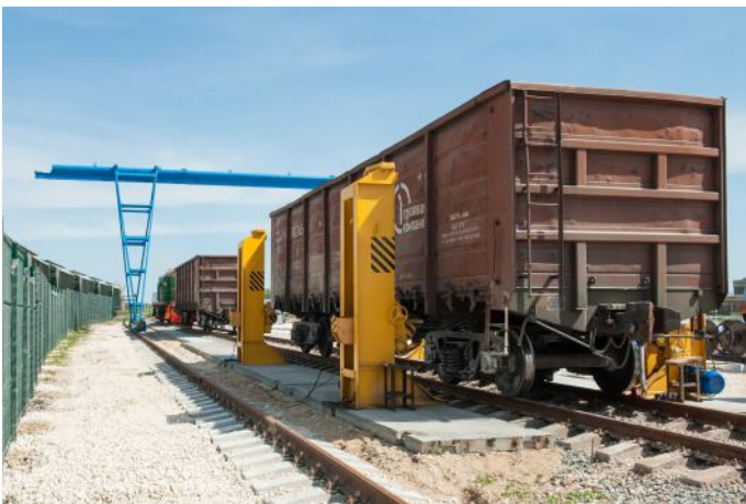
Stationary jacking unit — 160 ton capacity
