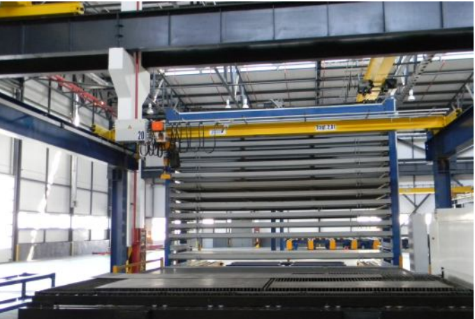
Automated sheet metal storage system
