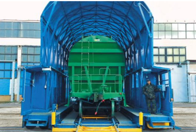
Traverser for freight car transfer with a load capacity of 60 tons
