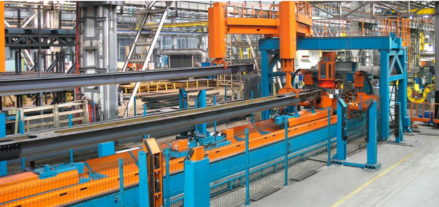
Automated complex for drilling of freight wagon centre sills (2 drilling gantries)
