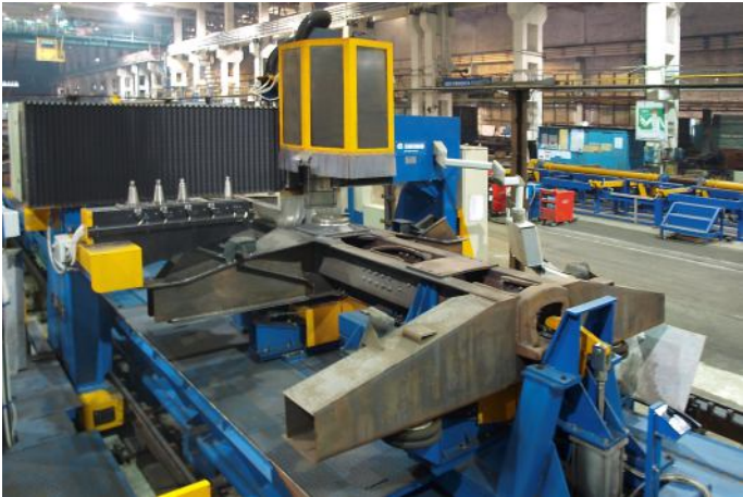
Automated complex for drilling of freight wagon frames
