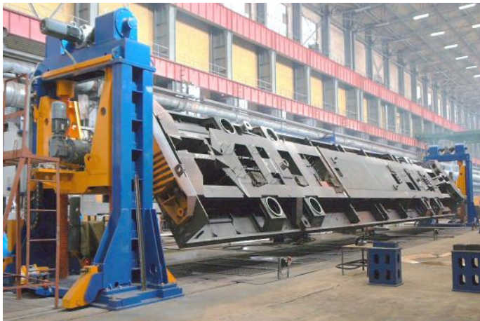
Headstock and tailstock positioners, load capacity 30 tons
