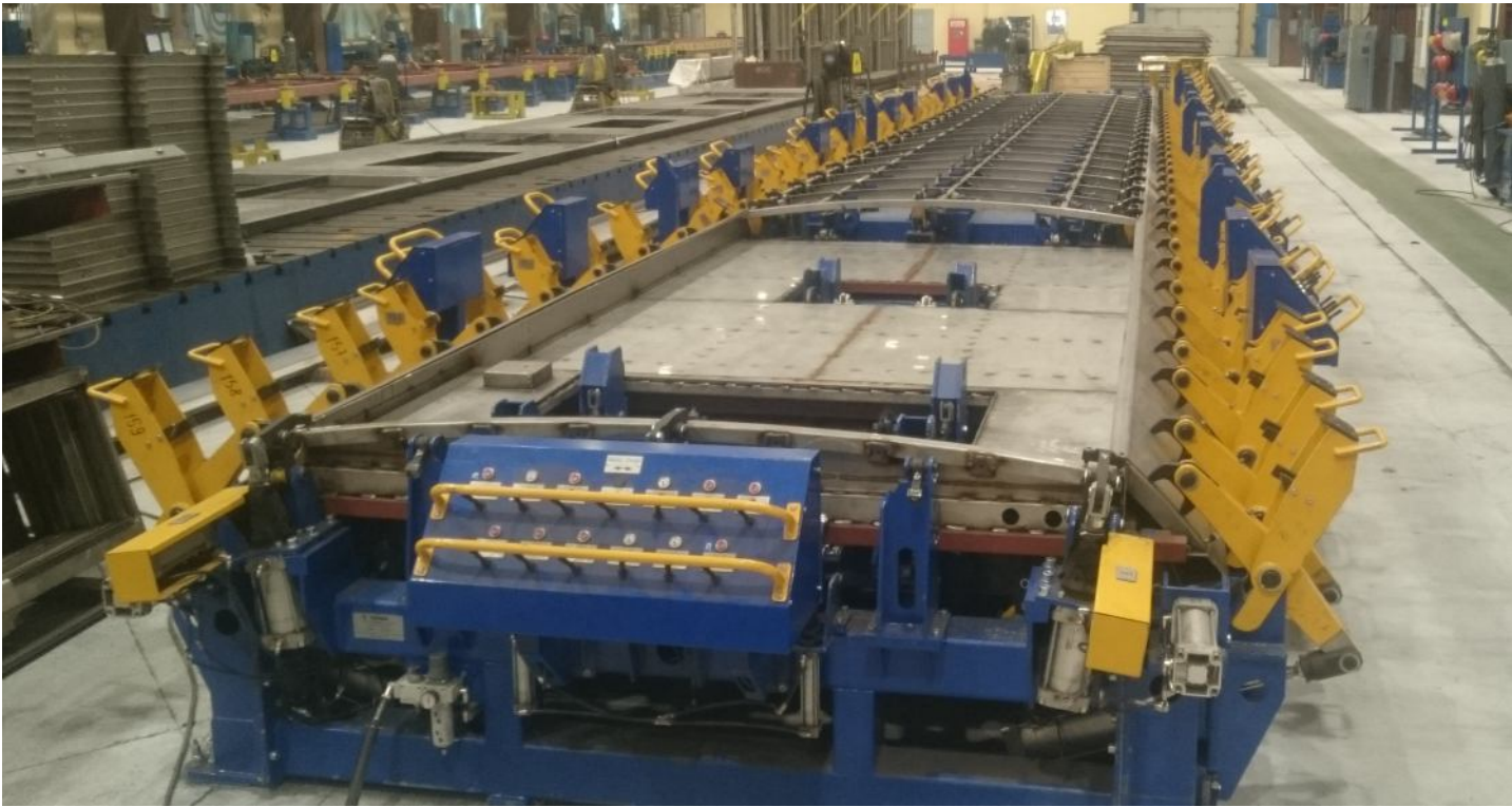
Multipurpose stand for metro wagon roof assembly
