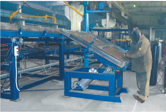
Hatch cover welding positioner
