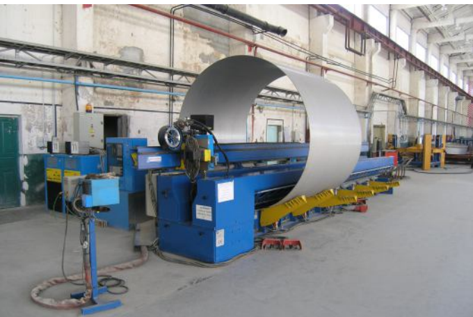
Stand for welding tank shells
