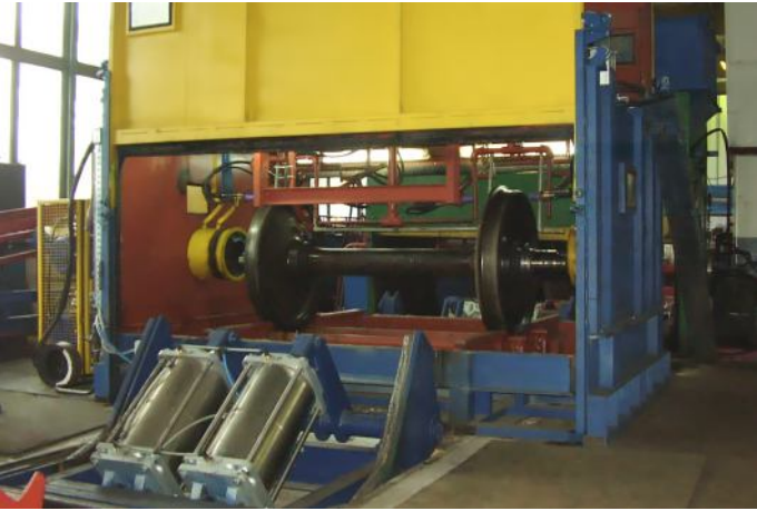
Automated wheelset cleaning system
