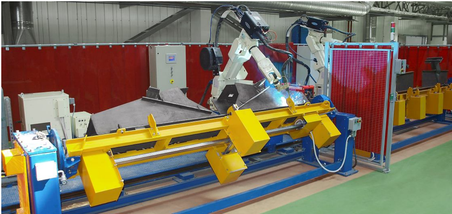
Robotic center for welding of cross beams
