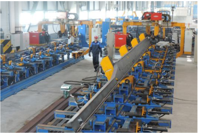
Automatic welding stand for variable cross-section I-beams
