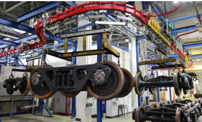
Suspended conveyor system
