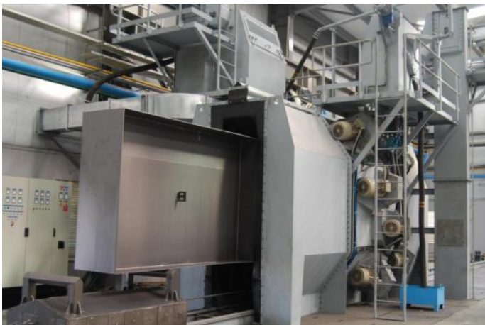
Shot blasting chamber for blast cleaning of welded metalwares
