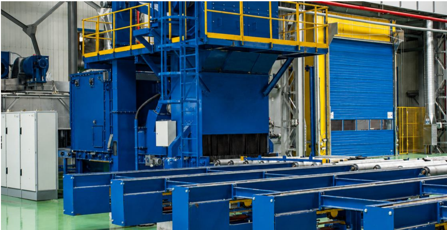
Shot blasting machine for cleaning sheet and profiled metal products
