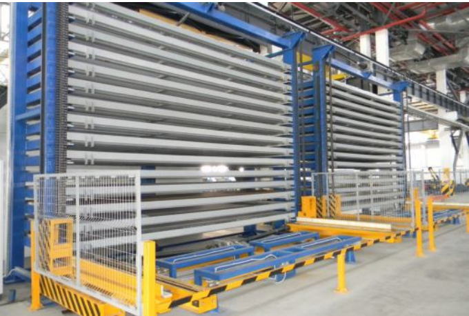
Automated sheet metal storage system
