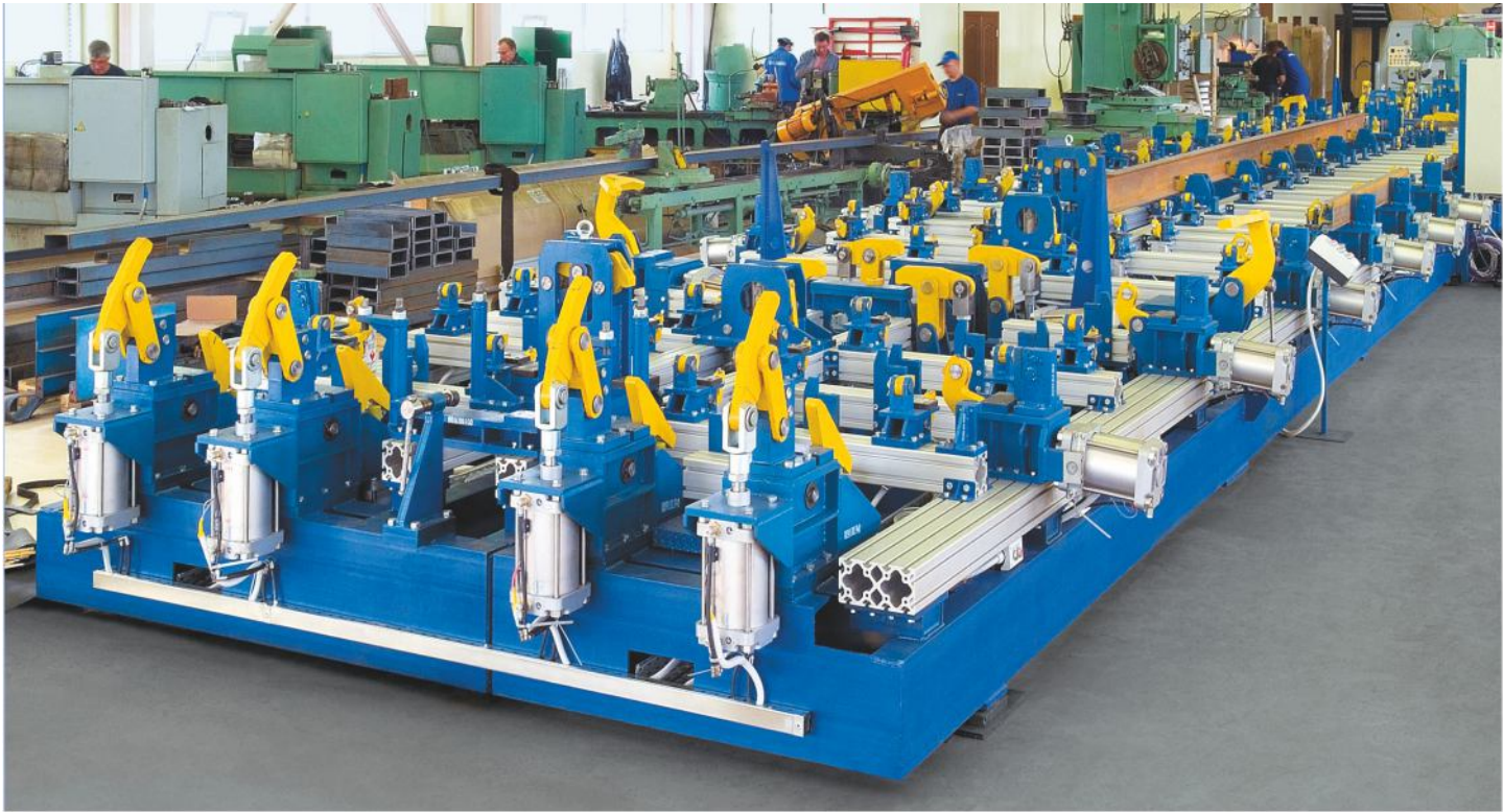
Multipurpose stand for assembly and welding of passenger wagon underframes
