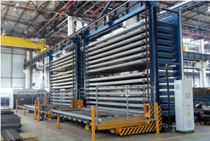
Automated sheet metal storage system
