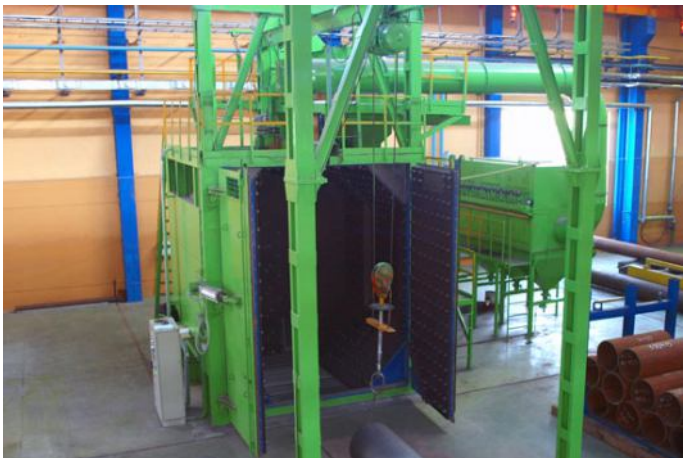
Shot blasting chamber with hanging workpiece
