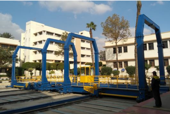
Traverser for electric locomotive transfer with a load capacity of 120 tons
