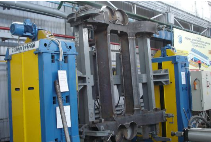
Headstock and tailstock positioners, load capacity 4 tons
