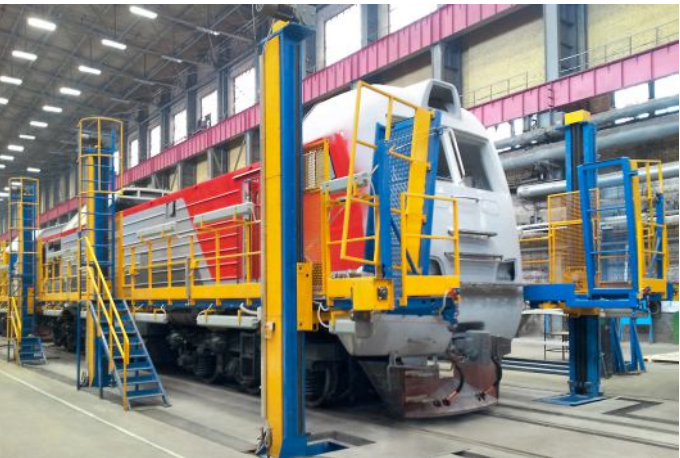
Elevated access platforms
