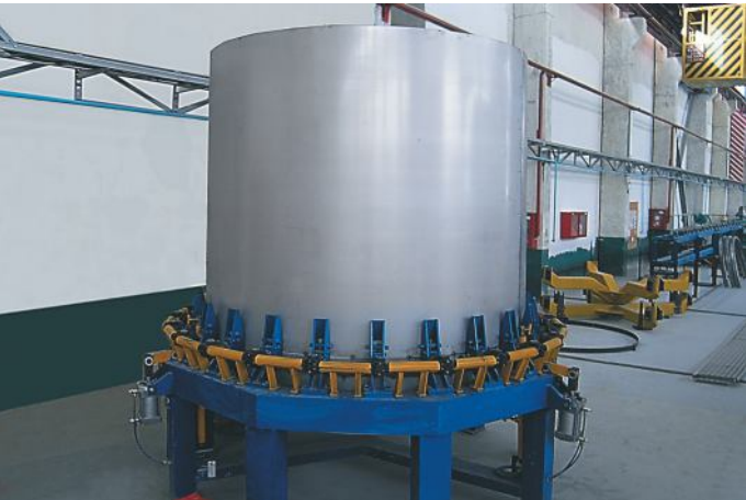
Tank shell-to-end cap assembly station
