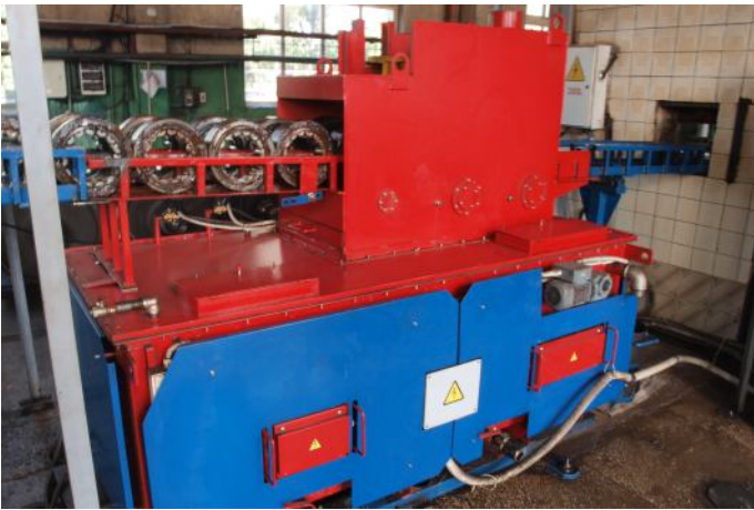
Bearing cleaning machine
