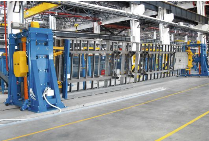
Headstock and tailstock positioners, load capacity 10 tons
