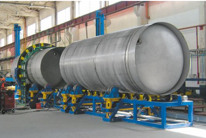
Tank shell assembly and welding line
