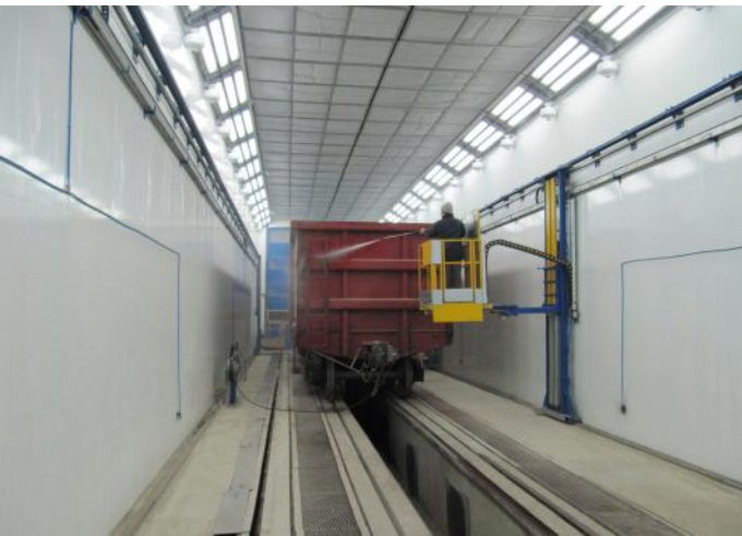
Painting and drying booth (with degreasing feature)
