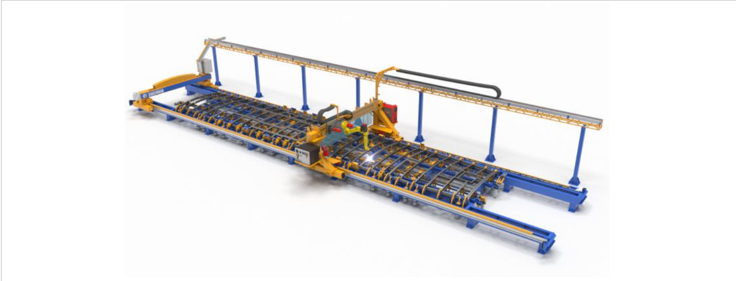
Robotic center for tram roof welding
