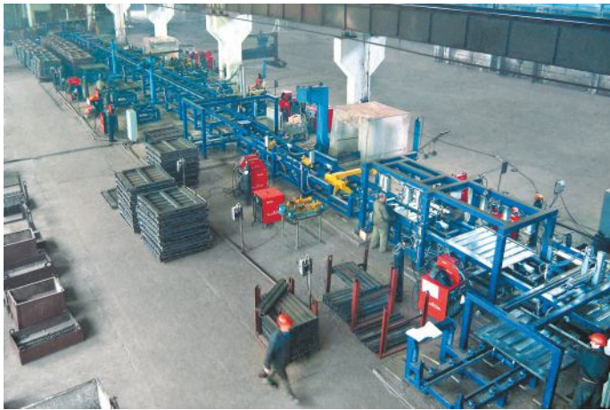
Gondola wagon hatch production line
