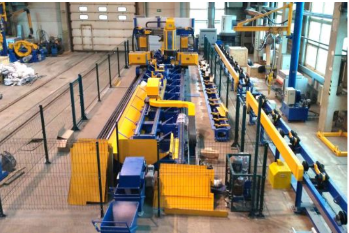
Automated complex for drilling of freight wagon centre sills
