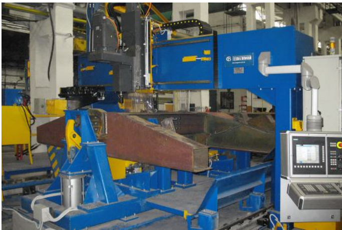
Drilling and riveting stand for underframes
