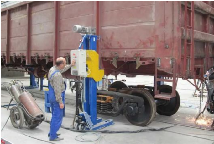
Mobile jacking unit — 28 ton capacity
