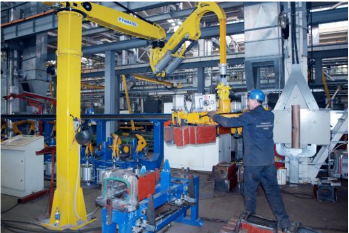
Assembly jig for center sills
