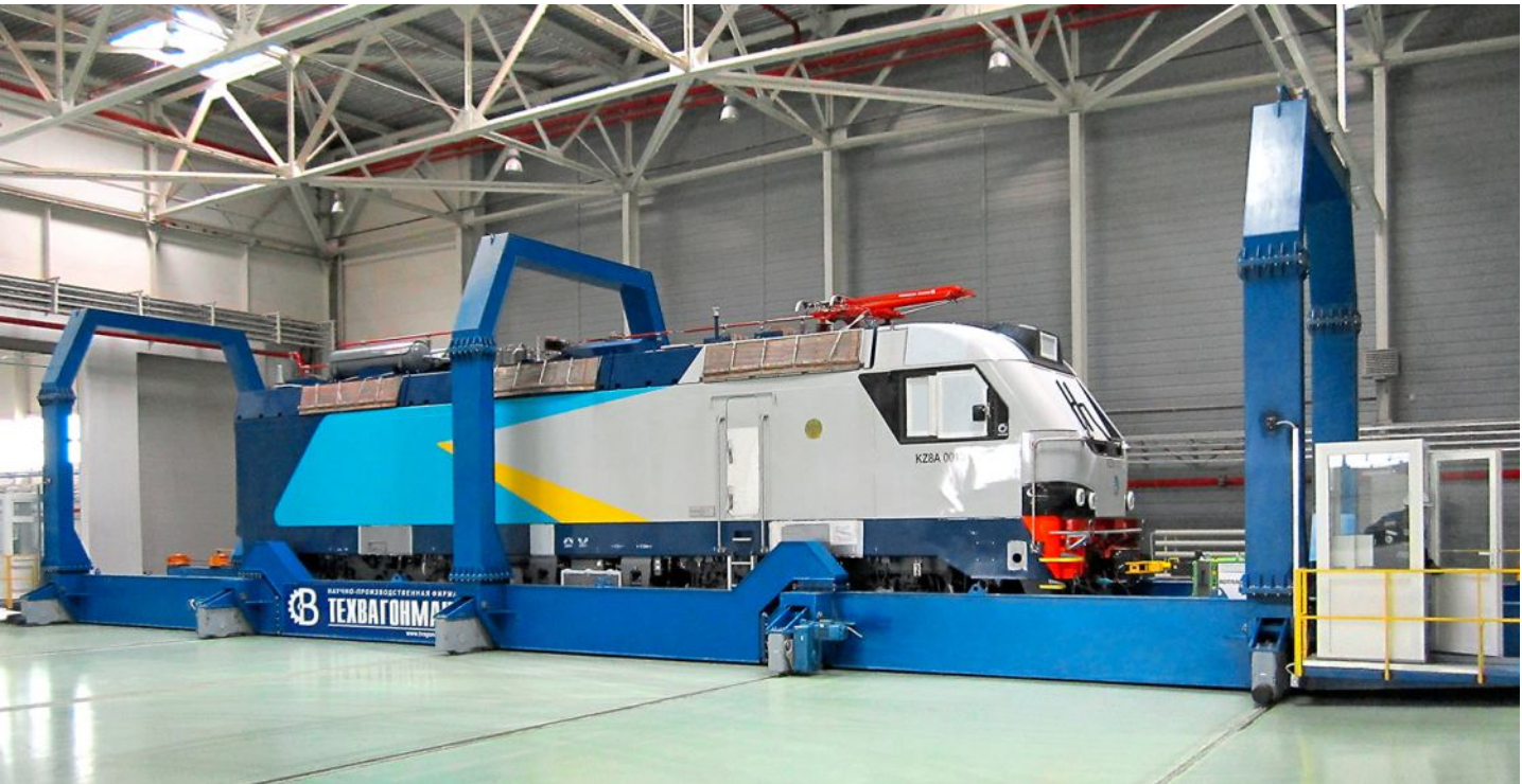
Traverser for electric locomotive transfer with a load capacity of 150 tons
