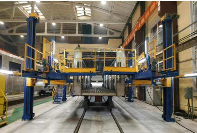
Elevated access platforms with side extension mechanism
