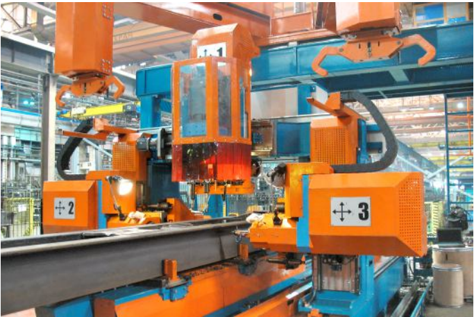
Automated complex for drilling of freight wagon centre sills (drilling gantry)
