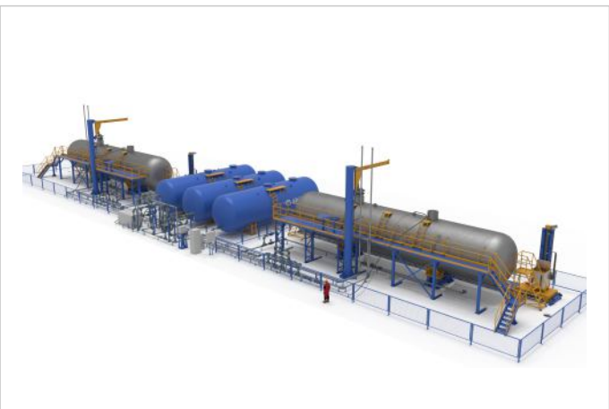
Stand for hydraulic and pneumatic tests of tanks
