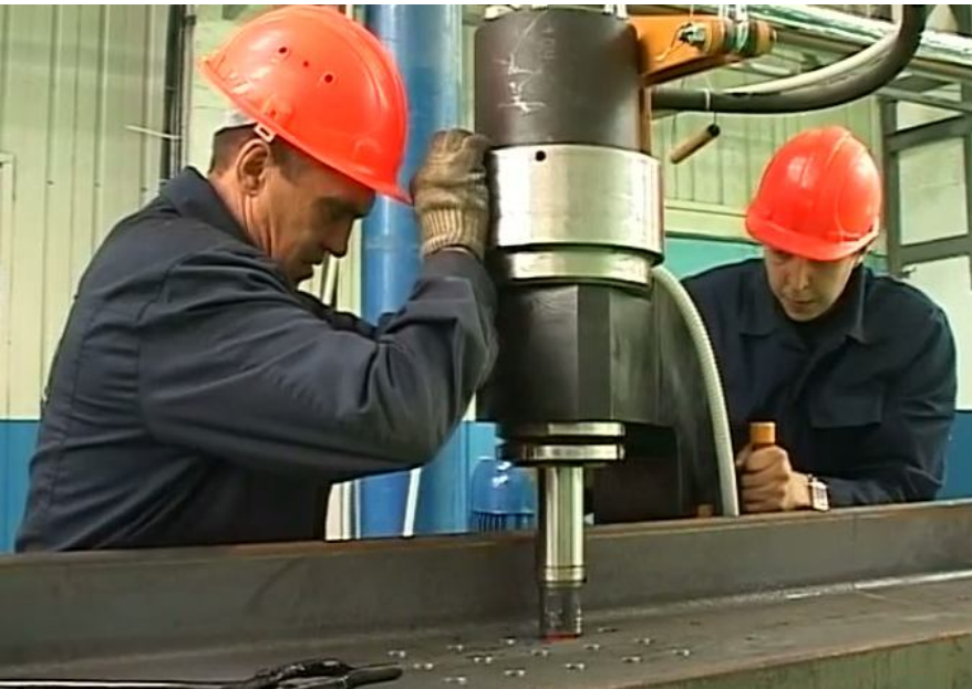
Center sill riveting plant
