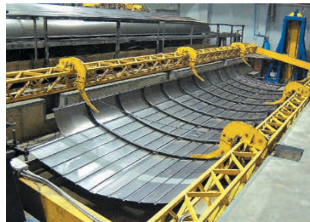
Positioner with vertical lift for passenger cars roofs welding
