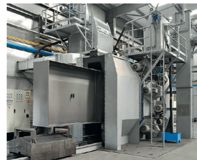
Shot blasting chamber for welded structures blast cleaning
