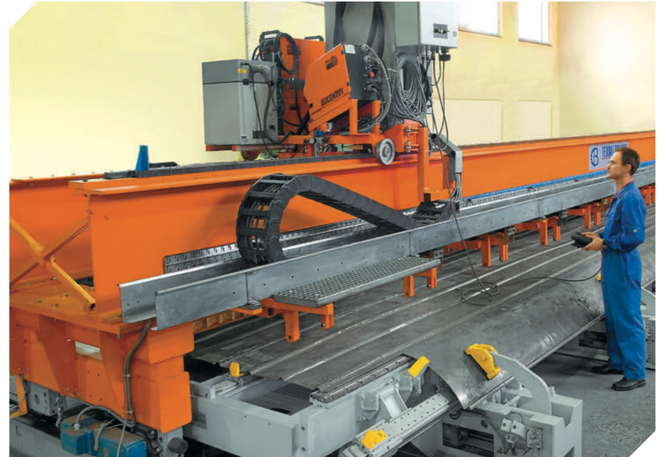
Multipurpose stand for passenger car roofs assembly and welding
