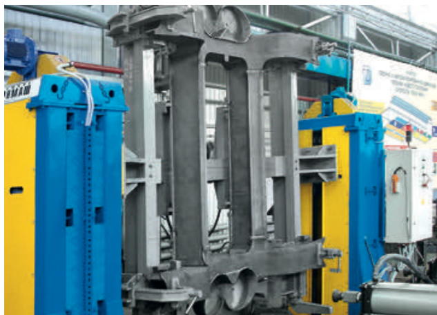
Positioner with vertical lift, load carrying capacity 4,5 t
