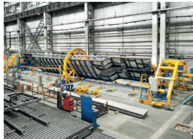
Positioner stand with vertical lift and a support ring (for long and non-rigid products)
