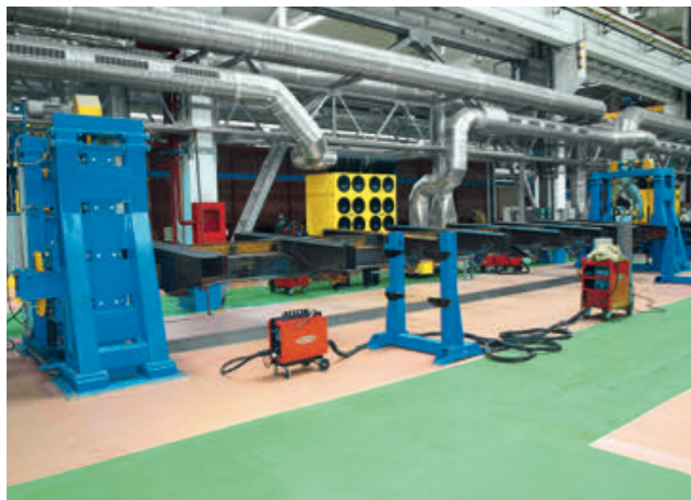
Positioner with vertical lift, load carrying capacity 15 t
