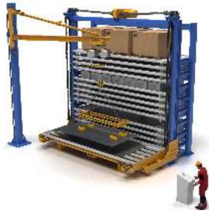
Sheet metal storage system with unit loads storage capacity
