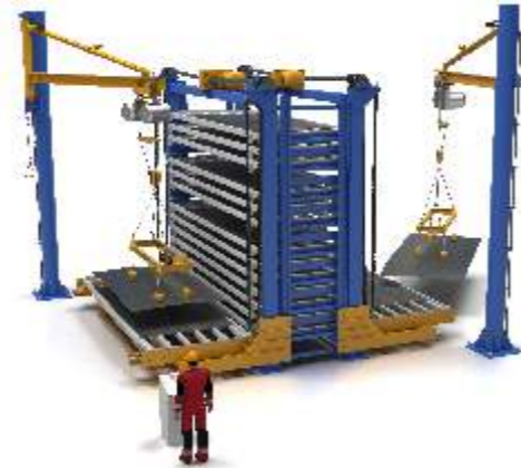
Sheet metal storage system with double-sided loading
