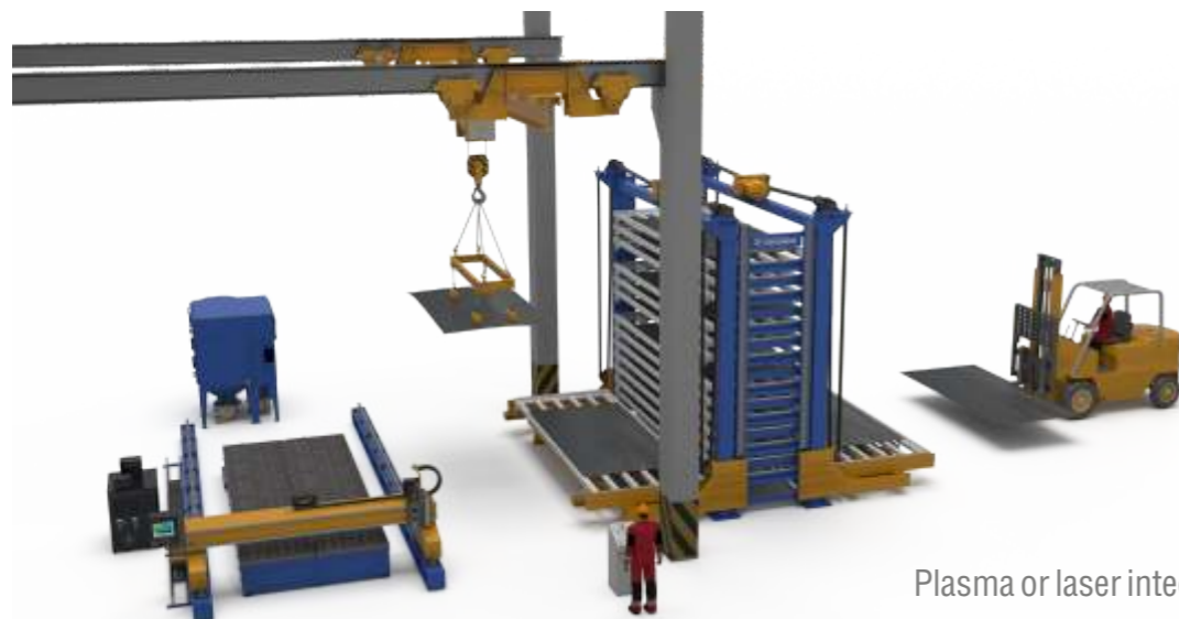
Sheet metal storage system with unit loads storage capacity
